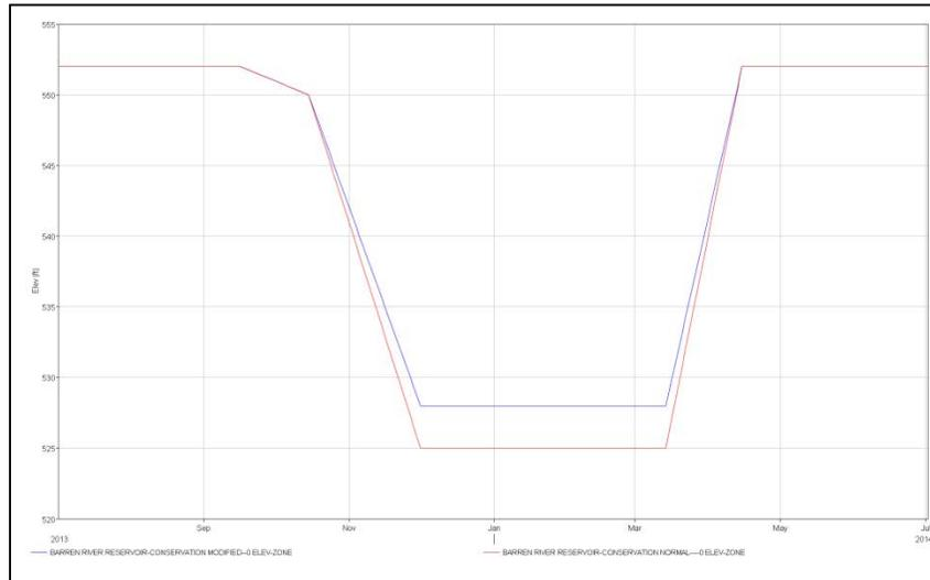
**Figure 2.2: Barren Reservoir Guide Curves as modeled**
