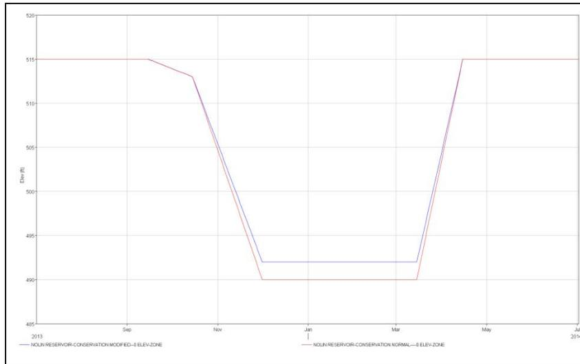
**Figure 2.4: Nolin Reservoir Guide Curves as modeled**
