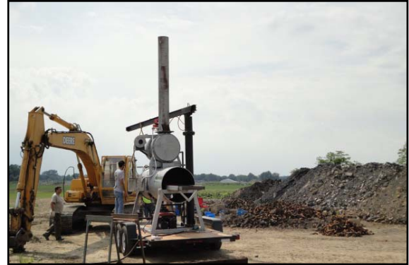
Thermal Flash Unit used to inert in-tact M74 bomblets.
