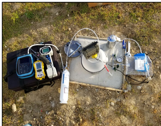
Exterior soil gas probe sampling (Jacobs stock photo).
