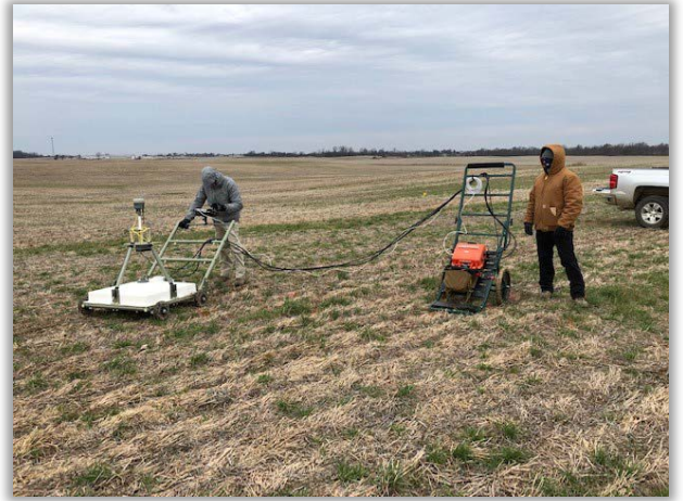
Use of Advanced Geophysical Sensors at the site (Metal Mapper 2x2)
