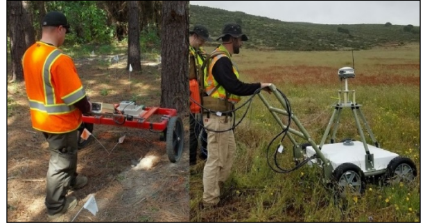
Geophysical instrumentation: Geonics EM61-Mk2 (left), Geometrics Metal Mapper 2x2
