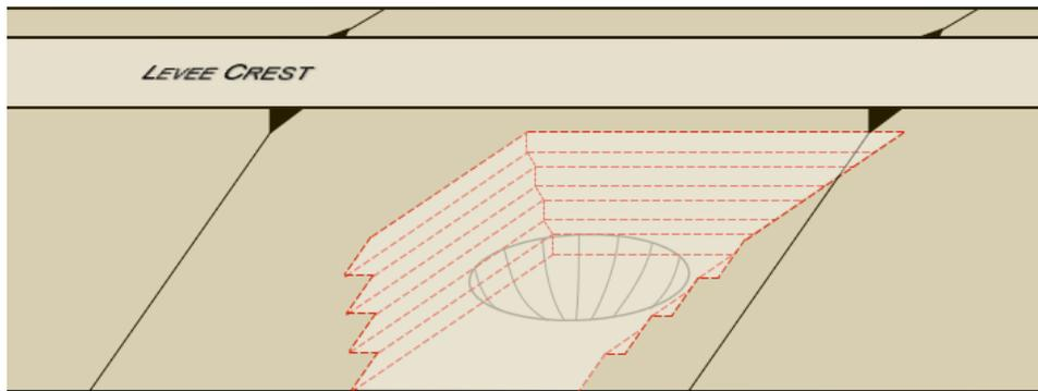
Figure 4: The area surrounding the rootball hole is benched in preparation for engineered fill.
